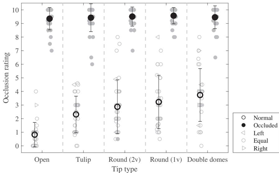
Fig. 4. Individual occlusion ratings (gray) and mean  $\pm$  1 SD (black). Circles indicate equal amounts of occlusion on both ears, triangles point in the direction of stronger occlusion.
