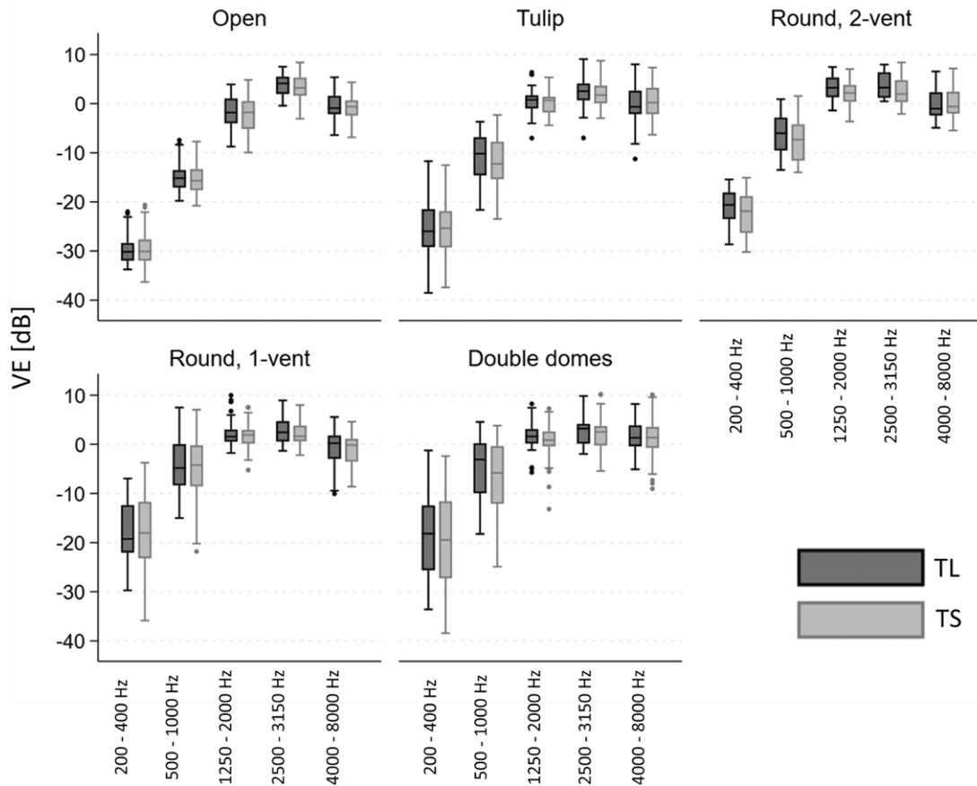
Fig. 6. Box plots for the VE after tip insertion by the test leader (TL, dark gray) and the test subject (TS, light gray). For clarity and statistical analysis, the measured VE spectra were averaged in five frequency bands. VE indicates vent effect.
