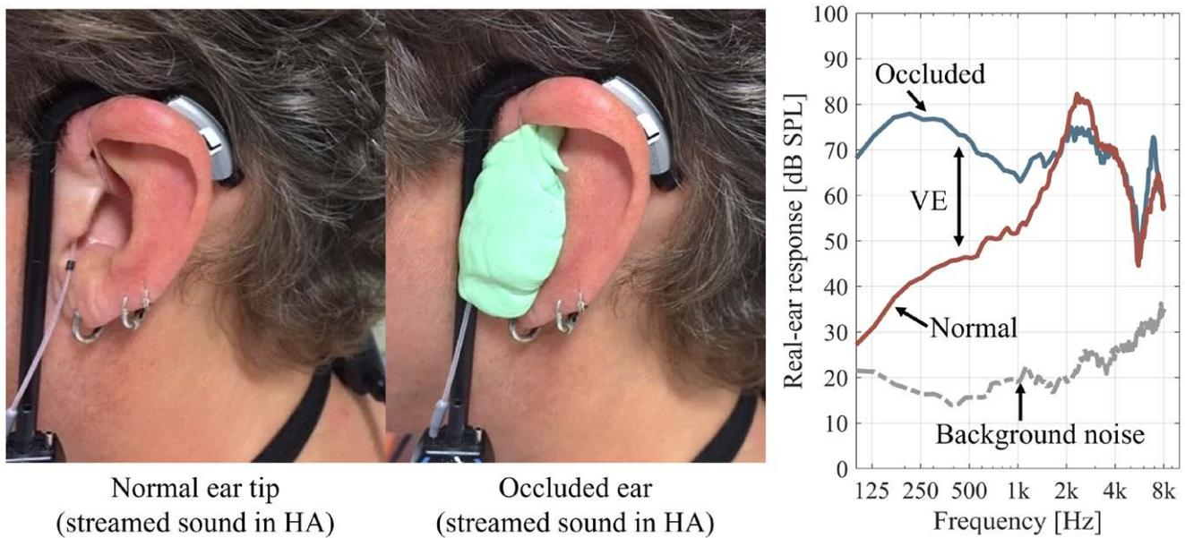
Fig. 2. VE estimation method. Responses were measured with brown noise streamed to the HAs both normally and with the ear occluded with impression material. The VE was computed as the difference between the two responses (normal – occluded). The dash-dotted line in the right panel represents the background noise inside the room as measured by the probe microphone inside the ear canal. HA indicates hearing aid; VE, vent effect.
