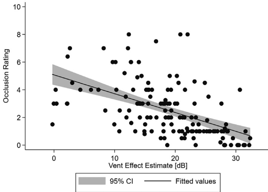
Fig. 5. Correlation between the VE estimate in the 315-Hz 1/3-octave band and the perceived occlusion. The two measures showed a significant correlation ( $p < 0.0001$ ) with a Spearman's rho of  $-0.61$ .
