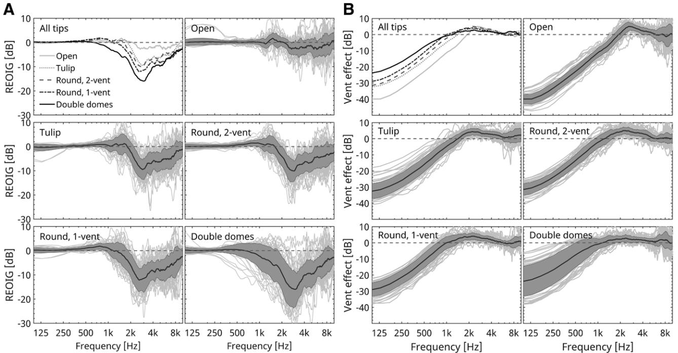
Fig. 3. A, Average REOIG across 58 ears for the five ear tips (top left) and (B) average VE across 58 ears for each ear tip (top left). The remaining panels in each sub-figure show the average REOIG or VE per tip (thick line) +/- one standard deviation (shaded area). The light gray lines represent individual measurements. REOIG indicates real ear occluded insertion gain.
