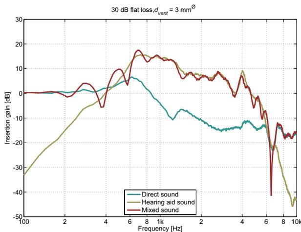
Figure 10. An example of the mixing of the insertion gain and the directly transmitted sound at the eardrum.
