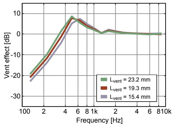
Figure 4. Vent effect as function of frequency for different vent lengths. An increase in length results in a decrease in low-frequency gain reduction and a shift of resonance frequency to a lower region. A vent diameter of 2 mm is used in the example. Reproduced from Kuk & Nordahn, 2006.
