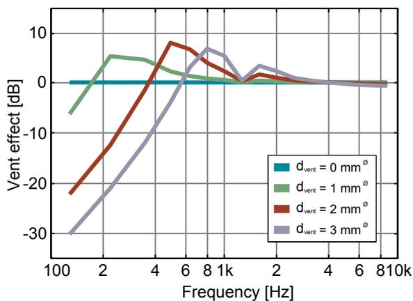
Figure 3. Effect of vent diameter on the output of a hearing aid. A 3 mm vent reduces the output at 200 Hz by as much as 23 dB compared to a closed earmould ( $\varnothing=0$  mm). Reproduced from Kuk & Nordahn, 2006.
