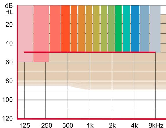
Figure 9. Example of a Sensogram measured with a 2.5 mm vent. According to the audiogram, the person has a 50 dB flat hearing loss. The Sensogram threshold is 60 dB for 125 and 250 Hz, however.
