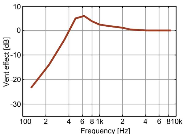
Figure 2. Vent effect in a hearing aid. Its shape is always the same with a resonance frequency at which sound is amplified, a frequency-dependent attenuation below the resonance frequency, and no effect above the resonance frequency.
