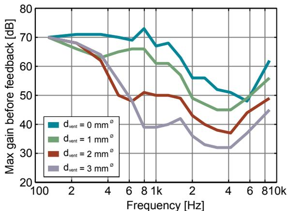
Figure 8. Maximum gain before feedback as a function of different vent diameters. As the vent diameter increases, the available gain decreases. The decrease is more rapid in the high frequencies than in the low frequencies. Reproduced from Kuk & Nordahn, 2006.
