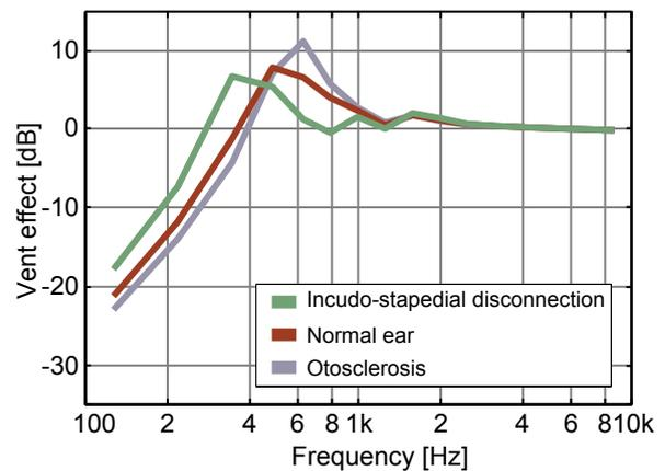
Figure 7. Simulated effect of middle ear compliance on the vent effect. The example is based on an earmould with a 2 mm vent diameter and a length of 19.3 mm. Reproduced from Kuk & Nordahn, 2006.
