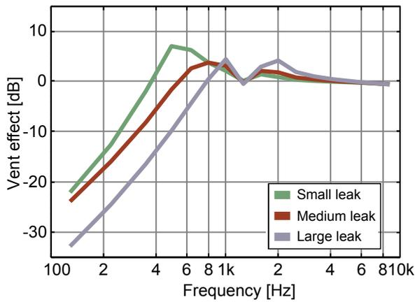
Figure 5. Effect of different degrees of leakage on the vent effect. The example is based on an earmould with a 2 mm vent diameter. Reproduced from Kuk & Nordahn, 2006
