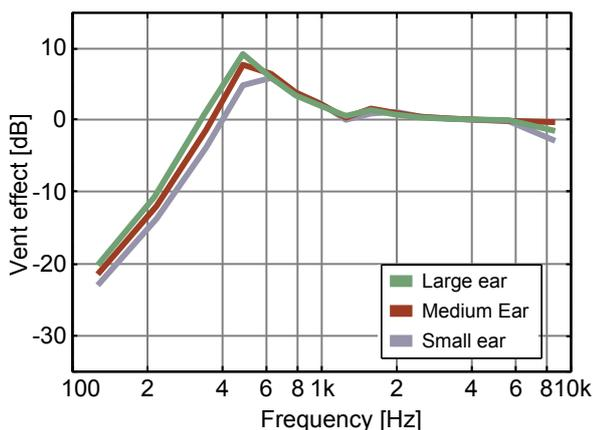
Figure 6. Effect of residual ear canal volume on the vent effect. The largest vent effect is seen with the small ear. The example is based on a vent with a 2 mm diameter and a length of 19.3 mm. Reproduced from Kuk & Nordahn, 2006.
