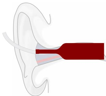
Figure 1. The vent and the residual ear canal function like a bottle.
