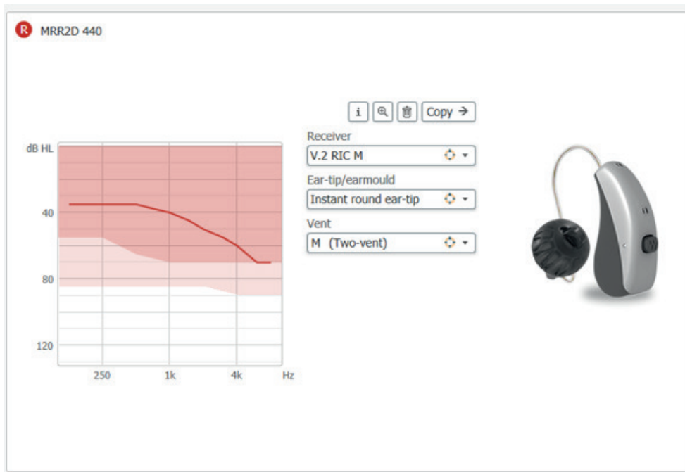
Figure 5 Acoustic Selection showing in Light Red: Maximum fitting range that the selected receiver (or tube, for BTEs) can give, it is the same as fitting ranges in the datasheets. Dark Red: Available fitting range for the entire system, including hearing aid and acoustic coupling.
