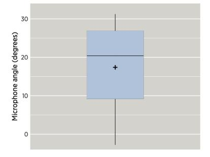
Figure 3: Distribution of microphone-angle measurements on 20 people wearing the Widex SmartRIC. The box represents the middle 50% of the data, from the first to the third quartile, with the line in between representing the median. The cross shows the mean, and the whiskers show the minimum and maximum values observed.
