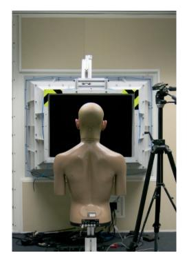
Figure 6: Measurement setup for wind noise, with the KEMAR positioned for wind from 0 degrees.
