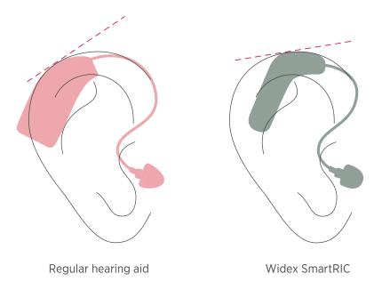
Figure 2: Stylized drawing of the microphone angle on the SmartRIC (right) compared with the larger angle often found on other RICs (left).
