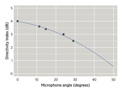
Figure 4: The relationship between microphone angle and directivity index. The dots represent measurements of microphone angle and DI, while the curve is a second order polynomial fit to the observed data.
