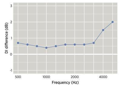
Figure 5: Difference in directivity index between the SmartRIC and the Moment mRIC, plotted as a function of frequency for the 1/3 octave frequencies from 500 Hz to 5 kHz. Positive values indicate a higher DI for the SmartRIC.
