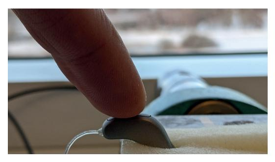
Figure 8: The SmartRIC subjected to a finger touch in the touch noise test. The SmartRIC was connected to an acoustic coupler and routed to headphones.
