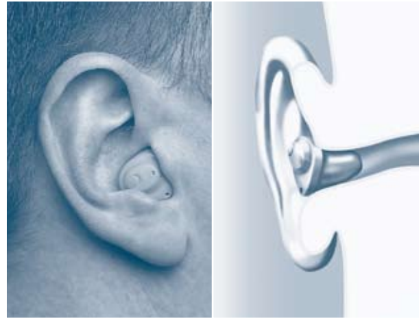
▶ Figure 6.02. An ITE hearing aid is a custom-made instrument that fits in the ear and is placed in the concha and ear canal.
