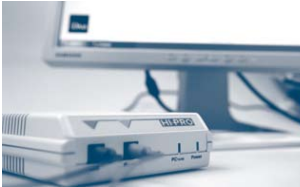
▶ Figure 5.08. A PC and a HI-PRO box. As the hearing aid is connected to the HI-PRO box, it can be programmed via the PC.
