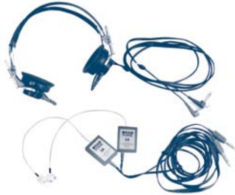
► Figure 4.04. There are different kinds of earphones available for measurement of air-conduction thresholds: supra-aural earphones that are placed on the ears (above) or insert earphones (below) which are inserted directly into the ear canal.
