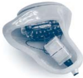
► Figure 9.14. A shell with a visible faceplate and electronics.
