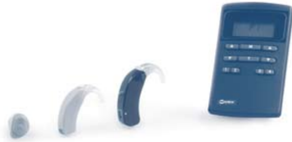
► Figure 5.07. The Quattro hearing aid from Widex was a programmable analogue instrument. Its four programs could be selected via a remote control.
