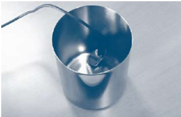
▶ Figure 8.25. Self-test; the hearing aid emits a sound signal and measures it through its own microphones. By analysing the signals picked up, it can detect faults.
