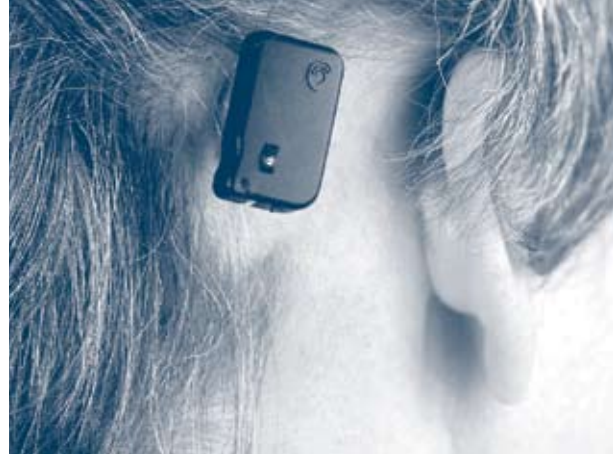
► Figure 6.09. A bone-anchored hearing aid is used where a person with conductive hearing loss will never be able to benefit from a conventional hearing aid.
