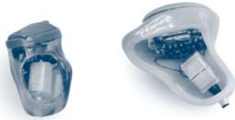
▶ Figure 7.04. Mounting of a faceplate in an ITE or ITC hearing aid.
