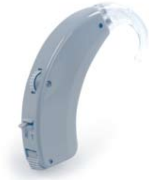
▶ Figure 5.05. Widex A1 hearing aid from 1972 with trimmer controls.
