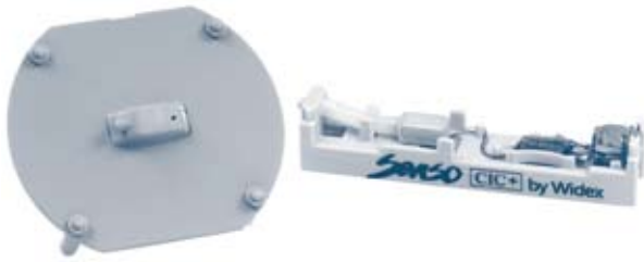
▶ Figure 7.03. As regards ITE and ITC instruments, a faceplate with the hearing aid electronics is supplied for installation in the shell. The electronics for CIC hearing aids come attached to a transport holder.
