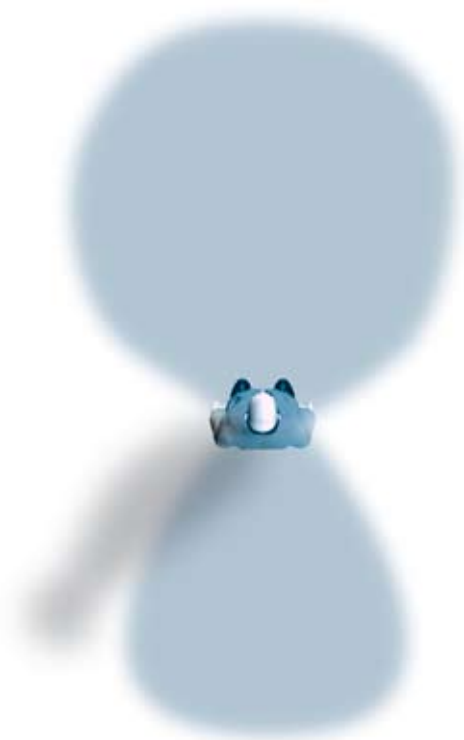
▶ Figure 7.08. A person seen from above. The blue colour indicates the area within which a directional microphone picks up sound.
