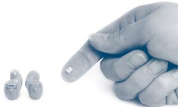
► Figure 5.12. Widex Senso in-the-ear instrument and chip. The chip is the “heart” of the hearing aid, because this is where signal processing takes place.
