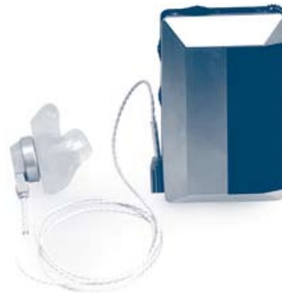
► Figure 6.05. A body-worn hearing aid. It consists of an earmould and the hearing aid itself, which is worn around the neck, in a pocket or on a belt.
