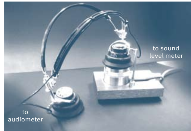
► Figure 4.18. The earphone is mounted on a coupler, and the audiometer is calibrated so that 0 dB HL corresponds to the RETSPL value for the different frequencies. The sound level meter measures the sound pressure in the coupler.
