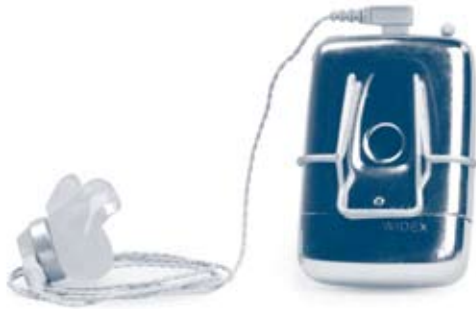
▶ Figure 5.03. Widex 561 body-worn hearing aid from 1956. The microphone, amplifier and batteries are encased in a box, and a cord conducts the amplified signal to a receiver clicked onto a custom-made earphone.
