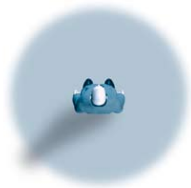
▶ Figure 7.07. A person seen from above. The blue colour marks the area within which an omnidirectional microphone picks up sound.
