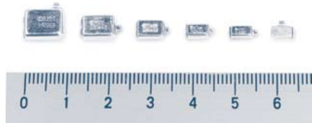
▶ Figure 7.21. Hearing aid receivers placed on a ruler. The larger the receiver, the higher the maximum output level.
