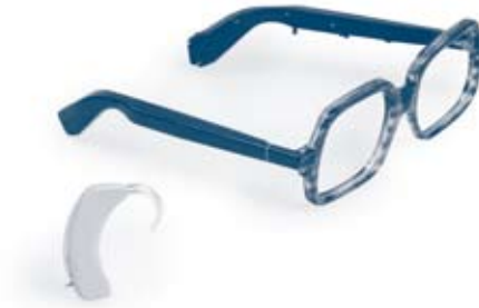
▶ Figure 5.04. Widex' first behind-the-ear hearing aid and a spectacle hearing aid from around 1960.
