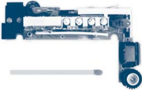
▶ Figure 7.14. Hearing aid amplifier with discrete components.
