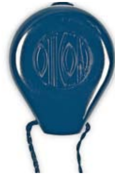
▶ Figure 5.02. Hearing aid with a vacuum tube amplifier. The hearing aid was powered by two batteries.
