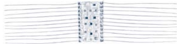
▶ Figure 7.15. Thin-film amplifier for a hearing aid. It is manufactured using a photographic process.
